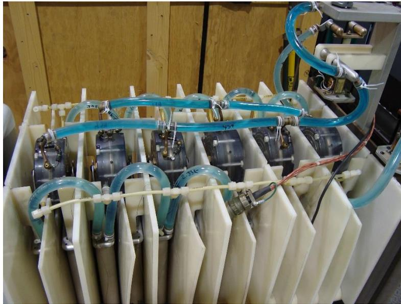
**FIGURE 6.** Mini-Marx system used to trigger the main Marx bank.
