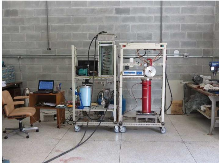
**FIGURE 7.** Experimental Rankine workbench to gather TPMF parameters [11].
