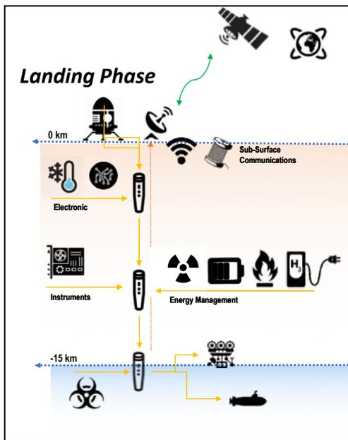
**Fig. 1.** Cryobot mission phases. The *Surface Phase* releases the probe into the ice and establishes DTE communication. The *Ice Descent Phase* operates the probe, communicating with the surface. The *Ocean Access and Mobility Phase* enters the ocean and deploys a science platform, working under strict planetary protection protocols.
