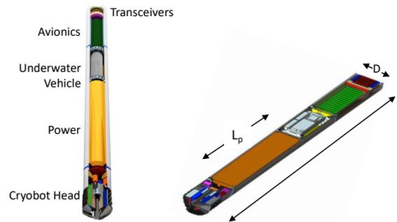
**Fig. 2.** Notional schematic of Cryobot systems. The probe diameter is  $D$ , the length is  $L$  and the length of the section for the power system is  $L_p$ .
