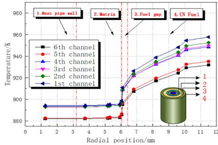
Fig. 8 Radial temperature distribution in different channel
