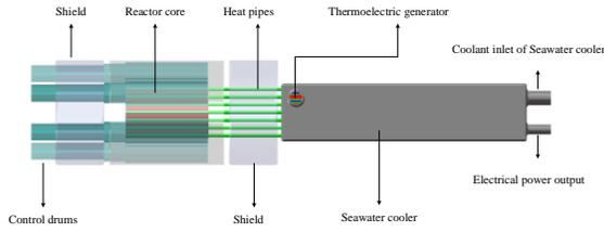
Fig. 1 Structure of micro nuclear reactor power source
