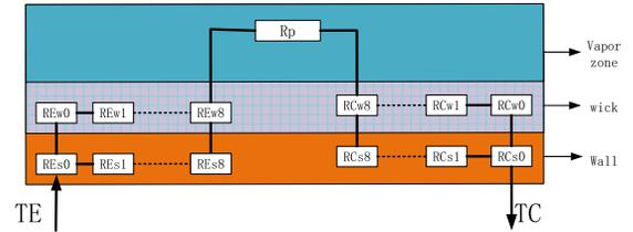
**Fig. 6** Heat pipe heat resistance diagram
