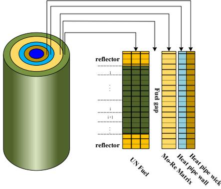
**Fig. 5** The radial control volume of the fuel cell equivalent
