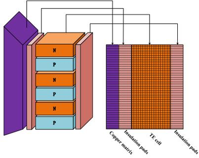
Fig. 7 Schematic of thermoelectric conversion model
