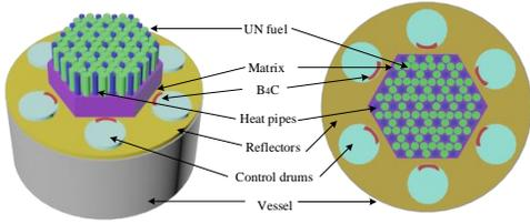
Fig. 2 Structure of HRP reactor core
