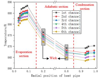
Fig. 10 Axial normalization heat pipe temperature distribution in different channel
