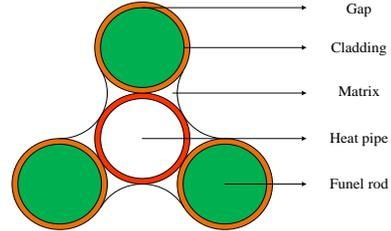
Fig. 3 A schematic view of the fuel unit
