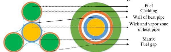
Fig. 4 Schematic of the fuel cell equivalent
