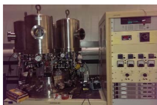
FIGURE 8. The copper test plate resides within the vacuum chamber bells jars, and is wired to an instrument rack for data acquisition and temperature control.
