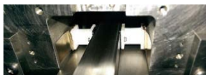
FIGURE 12. The heat source with the thermopile simulators and bonded metal flat springs being inserted into the EPD chamber.
