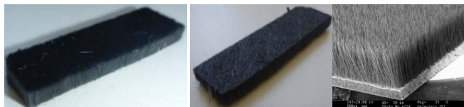
FIGURE 13. The carbon velvet thermal pad consist of carbon fibers (left) that are attached to a thin carbon sheet (center) which allow for excellent thermal contact while providing spring loaded compliance on a sliding interface.
