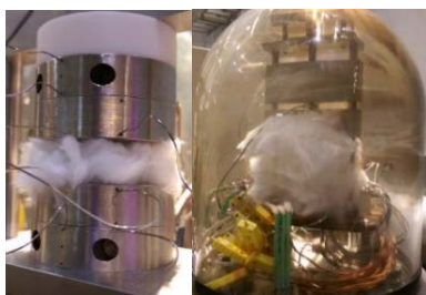
FIGURE 17. The TCRM fixture instrumented with high purity alumina cloth, and then placed under high vacuum inside a glass bell jar chamber.
