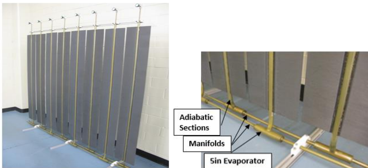
FIGURE 9. First cluster a) Actual radiator cluster b) Detail showing the manifolds, the heat pipe evaporators and adiabatic sections.
