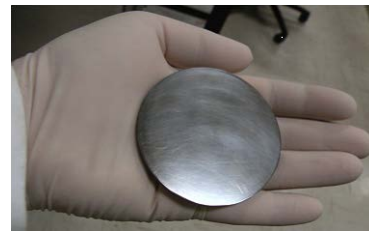
Figure 1. 63 mm diameter metallized p-type SKD puck fabricated at JPL
