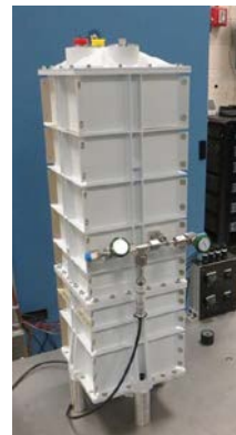
Figure 2. Aluminum Flight-like Housing for ASRG EU2 that will use ASC-E3 Pair 1.
