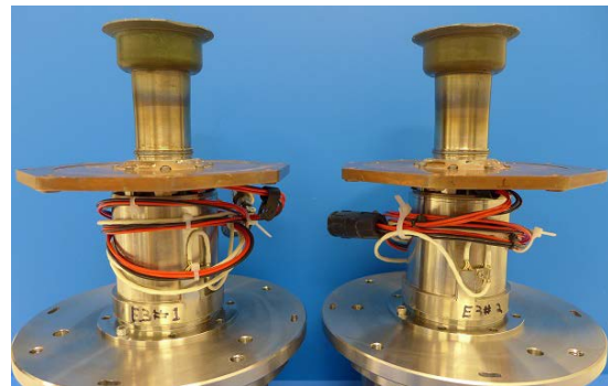
Figure 1. First Pair of flight-like ASC-E3 Engineering Unit.
