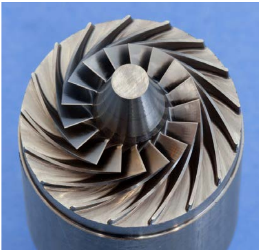
Figure 2. Ti6Al4V Compressor Impeller with Prototypical Aerodynamic Features
