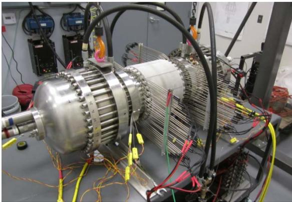
Figure 4 – PCU Test Setup (shown without insulation)
