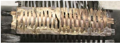
Figure 3. Test article braze joint
