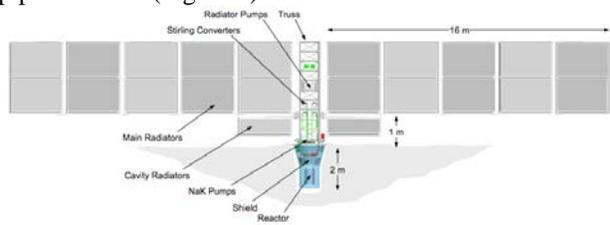
Figure 1. Fission Surface Power System
