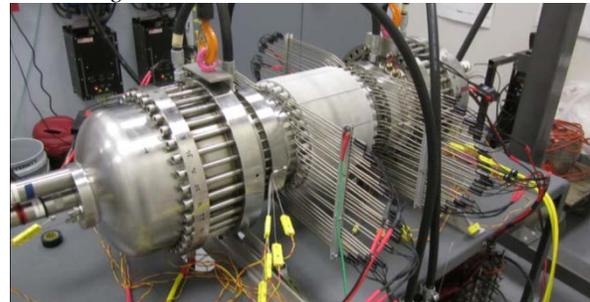
Figure 2. 12 kW Stirling PCU at Sunpower Inc.
