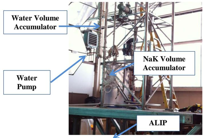
Figure 3. TDU Hot-End and Cold-End Sub-Systems being assembled at GRC
