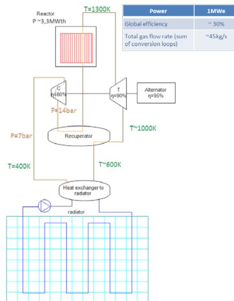
Figure 2 : thermodynamic map for reference cycle n°1
