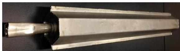
**Figure 4.** Filled 61 channel can ready for HIP.
