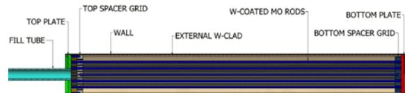
Figure 2. 61 channel HIP can design.
