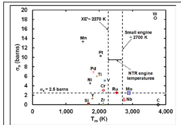
**Fig. 2.** Plot of thermal neutron absorption cross-section [6] against the absolute melting point.
