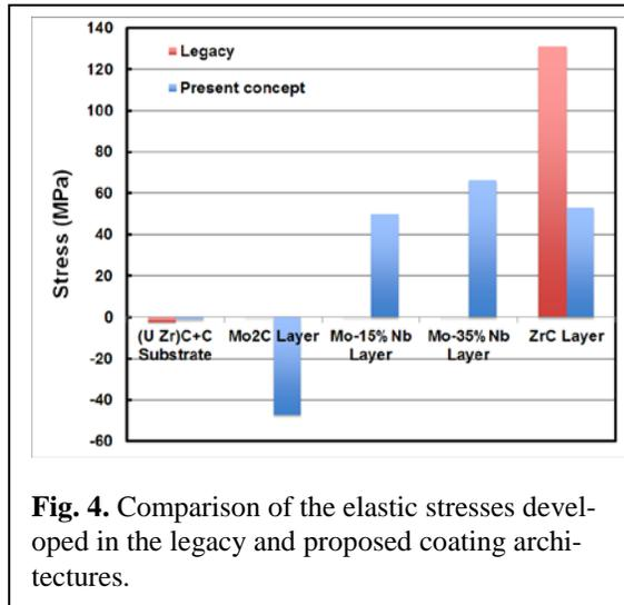
**Fig. 4.** Comparison of the elastic stresses developed in the legacy and proposed coating architectures.
