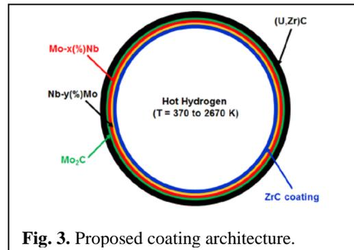
**Fig. 3.** Proposed coating architecture.
