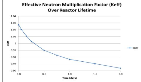
**Summary:** The current reactor design demonstrates the viability of the LEU-NRE concept for moving forward in NASA technology down-selection. Only minor modifications to the design are required for adequate lifetime.
