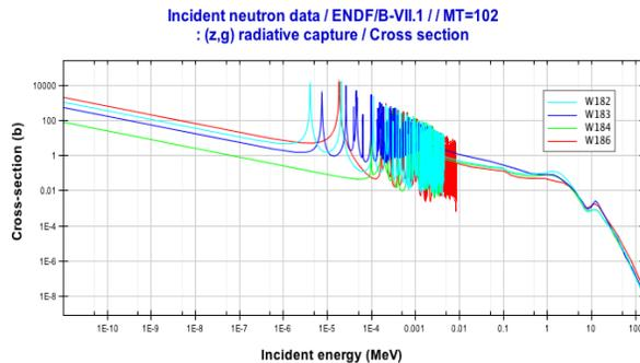
MCNPX 2.7 was used to determine various aspects of the neutronic characteristics of the NRE [4]. All of the calculations were performed in the “cold, clean” state. The <sup>184</sup>W enrichment was varied to determine the extent of enrichment that would be necessary for a tenable reactor design. The figure below demonstrates the necessity for enrichment with natural tungsten at the left extreme of the graph and fully enriched at the right-end.
