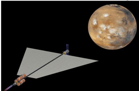
This spacecraft, which can be launched with a fleet of soon-to-be available SLS launch vehicles, is fueled primarily with hydrogen, and is fully reusable with no staging required. The reusable nature of this design enables a host of alternative mission architectures that more closely resemble an ocean voyage than our current piecemeal approach to exploration.
