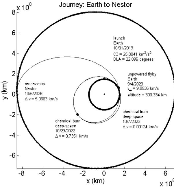
**Figure 1:** Trajectory generated from Earth to Nestor using EMTG. (The bold circular black line in the figure represent the trajectory of the Earth and Nestor)
