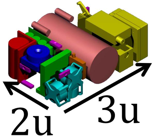
**Figure 2:** CAD model of a sample daughter CubeSat.
