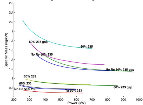
Figure 2: Specific Mass vs. Power for Many Reactor Configurations
