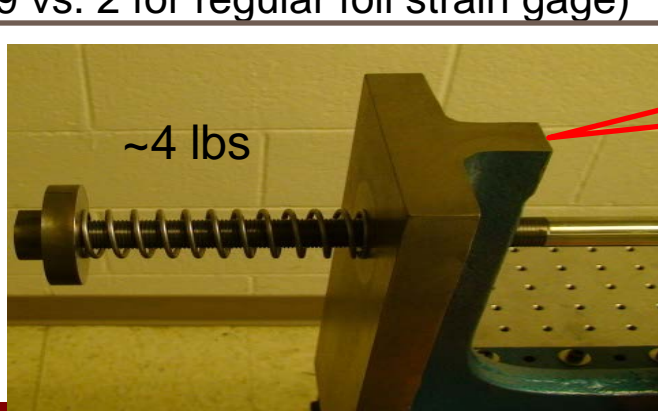
Semiconductor strain gages – specimen stress measurement (GF: 139 vs. 2 for regular foil strain gage)
