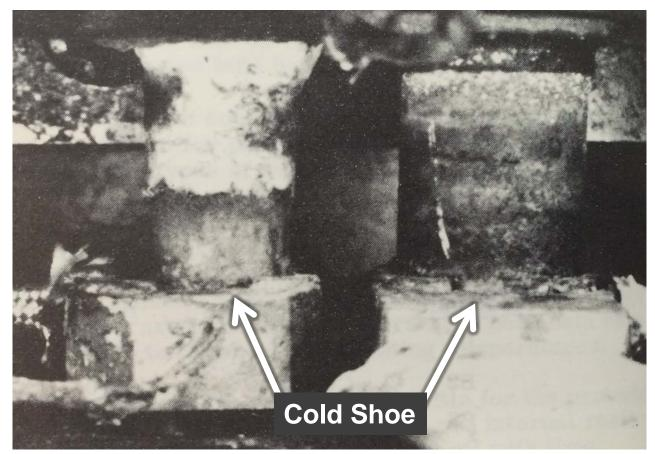
Ceramic Adhesive Coated Element after aging 5370 hours  $T_{hj} = 537^{\circ}C; T_{cj} = 149^{\circ}C$
