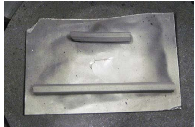
ORNL graphite composite samples after the final heat treatment to 2700 C. Long sample is a section from an extrusion run. Short one is run out material left over from extrusion run. (Heat treated to have some extra material)
