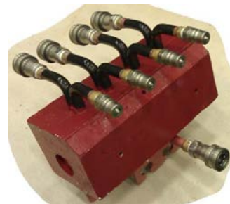
New Coil is Heavily Insulated and Rugged
