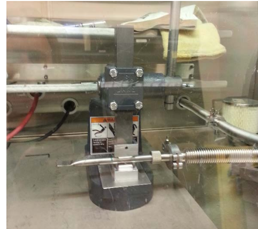
Crimp and sealing of W powder coated \text{UO}_2 sample in glovebox
