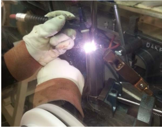
Images showing the 6" long 19-hole W-UO 2 HIP can assembly prior to, during, and after welding
