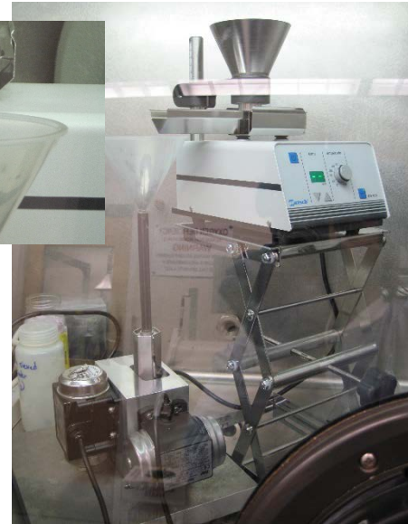
19 Hole HIP can W-UO 2 powder fill in glovebox
