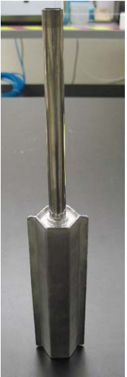
Images showing the 6" long 19-hole W-UO 2 HIP can assembly prior to, during, and after welding
