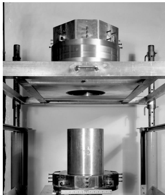
FIGURE 1. Vertical Assembly Machine and Disassembled Beryllium Reflected Core.
