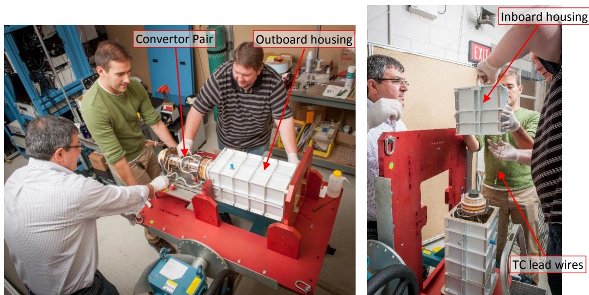
FIGURE 6. Converter pair situated for installation into the aluminum housing (left) and installation of inboard housing section (right).
