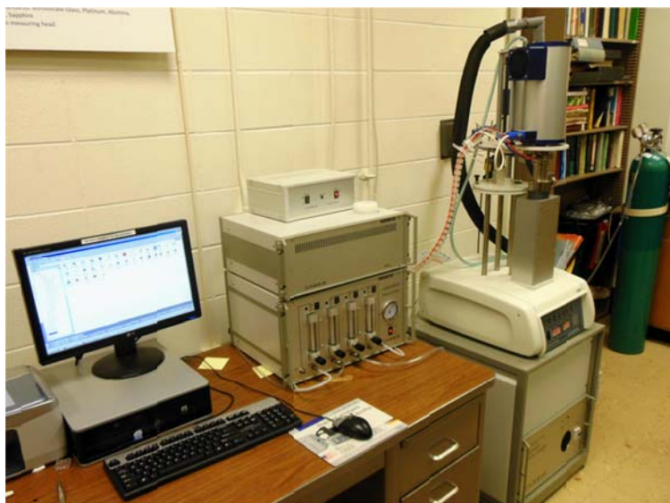
FIGURE 3. Linseis Messgeraete GmbH L75 Duel Push Rod Vertical Research Dilatometer System Showing the Location of the Various Major Components.
