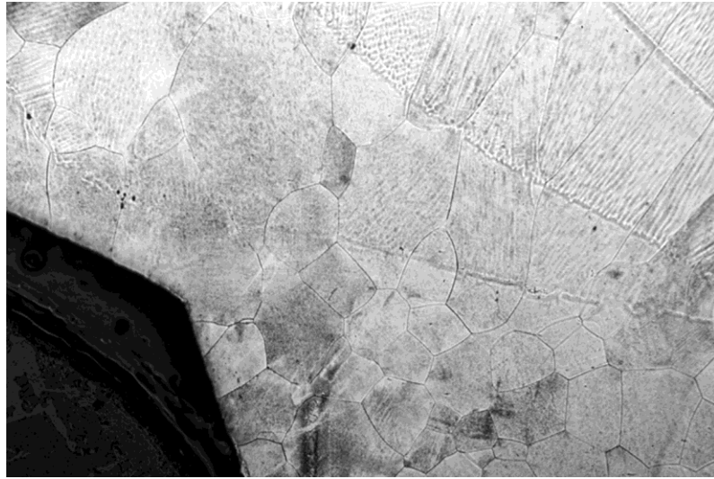
FIGURE 9. Metallography Microphotograph of a Strength Member Non-Anomalous Weld Heat Affected Zone with Part of the Weld Fusion Zone.
