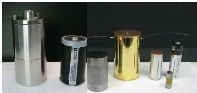
FIGURE 9. Watt and mW scale TPV System Hardware that has been developed, modeled and tested, D and AA size batteries for scale
