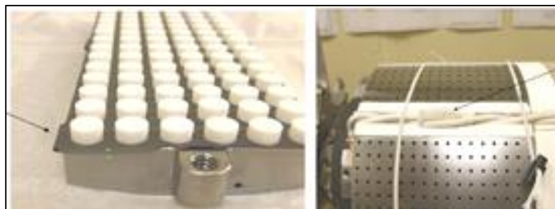
FIGURE 5. After Observing Shorts Inside the EU and QU, the MMRTG Flight Units Were Equipped with Additional Anodized Aluminum Plates (Left) and Deeper Wire Channels (Right).
