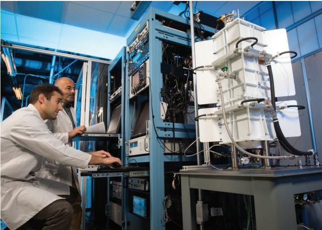
Figure 1. ASRG EU2 under test in NASA GRC's Stirling Research Lab.
