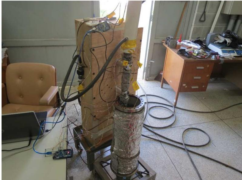
**FIGURE 5.** Shows the first experiment set of a cooper-water thermo-siphon performed in the end of 2016. The thermo-siphon must run in the vertical optimally because it does not have a wick inside the tube.
