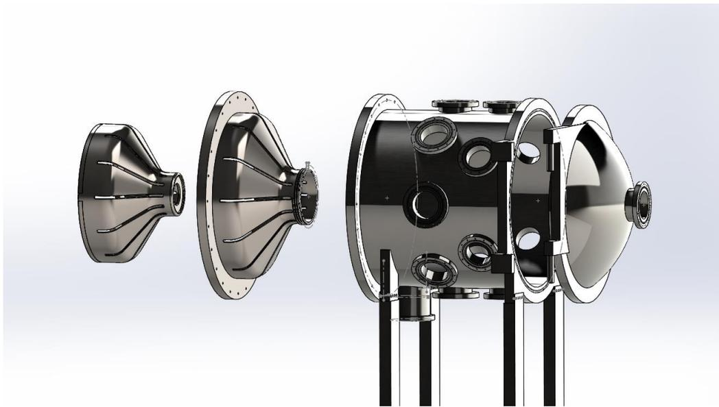
**FIGURE 8.** UAH MITL assembly, 10 ohm. Exploded view showing anode and cathode clearly.
