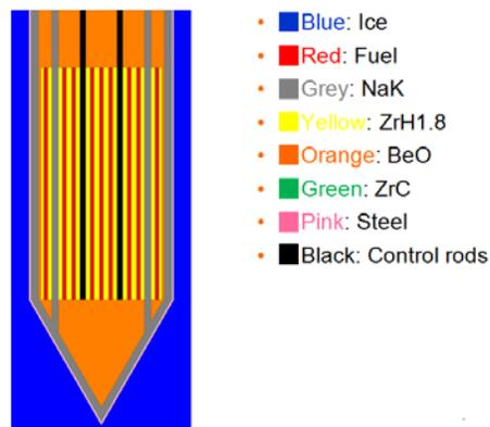
**FIGURE 3.** Vertical cross section of the LEU reactor.
