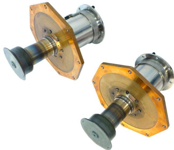
Figure 1- Completed ASC-E3 Pair 3 Convertors
